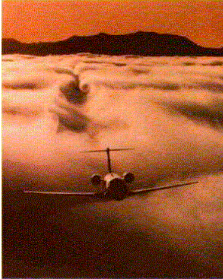
Fig 6 Downwash and wing vortices in the fog. (Photographer Paul Bowen, courtesy of Cessna Aircraft, Co.)
